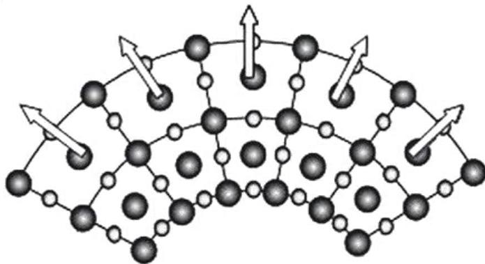
$$P_\alpha = \mu_{\alpha\beta,\gamma\delta} \frac{\partial \varepsilon_{\beta\delta}}{\partial r_\gamma}$$
