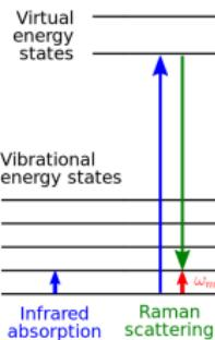
Stokes scattering : inelastic scattering of an *incident photon* interacting with a *phonon*.
